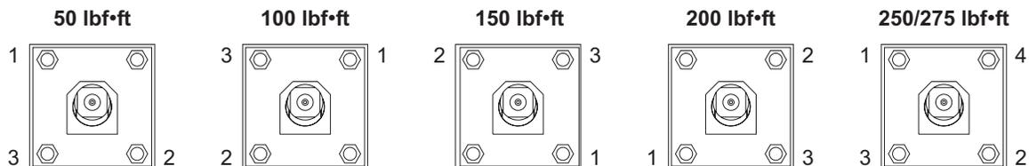
• Initially torque the hex nuts to 50 lbf•ft (68 N•m), then torque the hex nuts in increments of 50 lbf•ft (68 N•m) until 275 lbf•ft (373 N•m) is reached (repeat the last torque sequence to achieve 275 lbf•ft). Double check the final torque.
