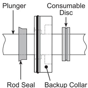
6. Slide the backup ring over the plunger and rod seal. Push the backup ring into the hydraulic end cap (this requires considerable effort). The rod seal will seat into the backup ring.
