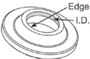
**The corner between the face of the cone and the inside diameter should be square and sharp. Use your fingernail along the edge. If you catch your fingernail on this edge, it is an indication of a bur, crack or chip; a bur can be removed otherwise replace the mini disk.**
