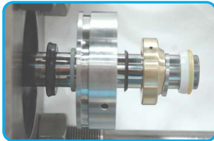
8. Slide a backup hoop and high pressure seal onto the plunger. Ensure the taper on the backup hoop faces the high pressure seal.
