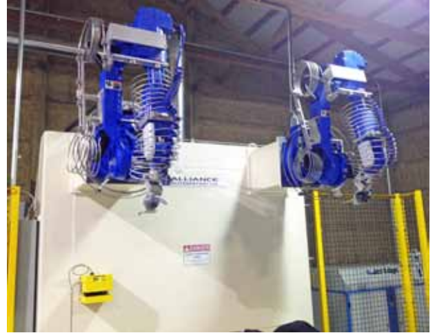
Alliance Automation's robotic waterjet system features dual wall-mounted robots and a sturdy frame ensuring consistent tight part tolerances. Photo credit: Alliance Automation, LLC
