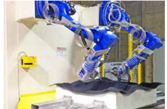
Alliance Automation's robotic waterjet trimming cells combine Motoman HP20D robots and Jet Edge's 60,000 psi iP60-50 waterjet intensifier pumps for industry-leading precision and dependability. Photo credit: Alliance Automation, LLC
