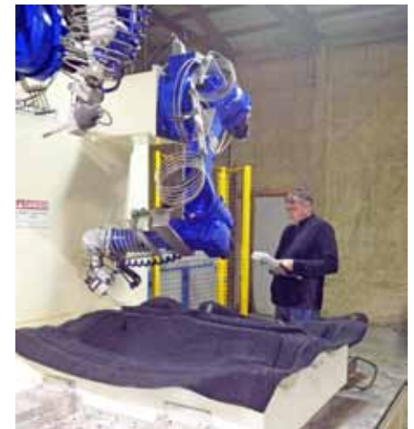
Alliance Automation's robotic waterjet trimming cell can be set up so that many different parts can be programmed and selected through the touchscreen HMI on the control panel. Photo credit: Alliance Automation, LLC.
