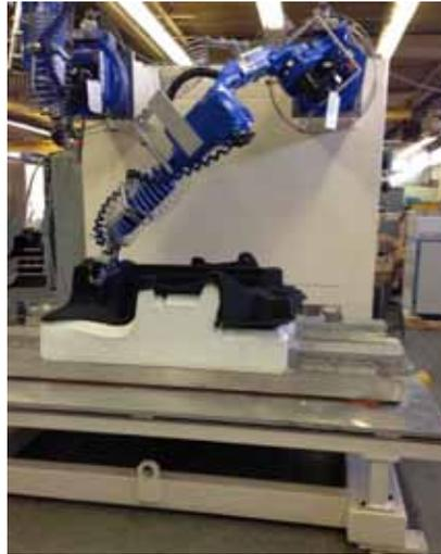
**Wall-mounted robots allow for the first 2 axis to be mounted forward, over the part. This feature allows for a larger work envelope and motion to work easier around larger shaped parts. The system includes a dedicated part holding nest that incorporates a vacuum to remove excess moisture and assist with holding the parts in place.**
